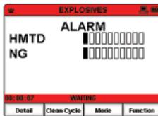
Color-coded display shows status of instrument. Green when ready, yellow when analyzing and red when a detection is made.
